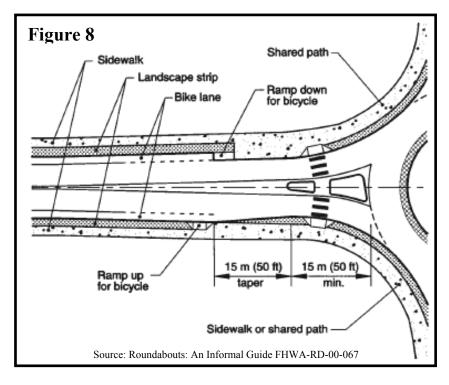
the approach to a Roundabout. Other options that angle the ramps between 30 and 45 degrees to the bike lane are gaining favor. Making these ramps of a different material than the sidewalks will help prevent visually impaired pedestrians from confusing the ramps as part of the sidewalk and walking inadvertently into the roadway. A selection of treatments for bicyclists can be viewed at a presentation at <u>http://www.teachamerica.com/roundabouts/RA055A\_ppt\_Moule.pdf</u>
