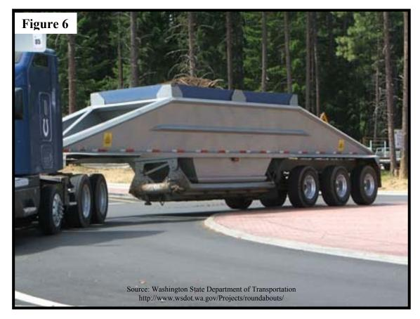
Since emergency vehicles are typically smaller than tractor trailer units, they are easily accommodated at Roundabouts, and because Roundabouts typically experience less delay and less queuing traffic, emergency vehicles are rarely delayed by traffic at Roundabouts.
