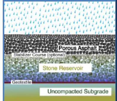
*Porous Asphalt Pavements with Stone Reservoirs.* Federal Highway Administration, April 2015.
