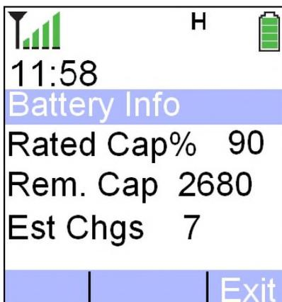
The APX 4000/6000 portable radios are designed to use Motorola IMPRES batteries. IMPRES batteries have a chip in them that communicates with the AC charger; this helps to recondition the batteries and negate "memory effect."
