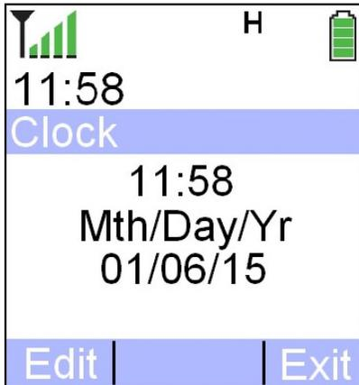
The APX 4000/6000 allows the user to change the day, date, and time of the radio. For instance, users can opt to use a 12hr clock or a 24hr clock. This option is selected by pressing the menu select buttons under the "Clck" tab on the radio's menu bar.
